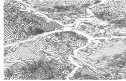
Microstructure of hyper eutectoid steel
