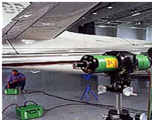
Figure 2. Detection of cracks in aircraft structure by Radiography method
