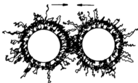
Figure 4. Schematic representation of steric stabilization.
